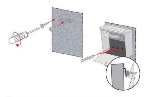
Using a masonry style drill bit(not provided), drill the bottom three pilot holes approximately 2 inches deep into the wall material. Now hang the Townhouse from the mounting bracket and secure to bottom using the three 21/4" screws provided. Be sure to put some weather resistant caulk into the holes...If your wall is a thick brick, stucco or concrete you will may need masonry screws or anchors for attachment, consult a contractor if necessary.
