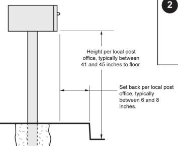
For 3" Round In-ground Post (item 7505, 7507, 7515 or 7516) or Standard In-ground Post (item 5525): Pour the concrete (at least 1 cubic foot recommended) completely around the post, making sure the post and mailbox are level and correctly positioned according to your local post office.
